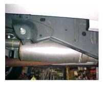
INSTALL MUFFLER # B ONTO HEADPIPE 1 ½" TO 2". USE CLAMP # E TO SECURE MUFFLER TO HEADPIPE. DO NOT TIGHTEN. USE A JACK STAND TO HOLD UP THE MUFFLER. MUFFLER INLET IS LOOKING INTO THE LOUVERS. OUTLET SHOULD BE AT T HE 10 O'CLOCK POSITION.
