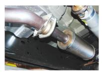
TO REMOVE YOUR STOCK EXHAUST, REMOVE IT FROM THE 2 BOLT FLANGE LOCATED JUST IN FRONT OF THE MUFFLER AND REMOVE HANGERS FROM RUBBER GROMMETS BY PULLING EXHAUST TOWARDS THE REAR OF THE VEHICLE, USE WD-40 TO AID IN REMOVAL, LEAVE GROMMETS IN PLACE.
